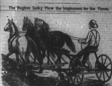
The important feature of having the plow located at the side of the Sulky instead of behind and between the wheels, as is the case IN ALL OTHERS, is controlled by the HUGHES patent, and example the applied by other manufacturers.
